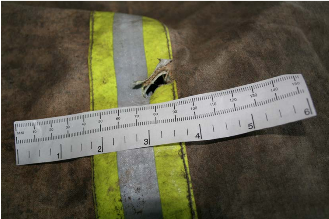
Penetration site of right leg of over-trousers
