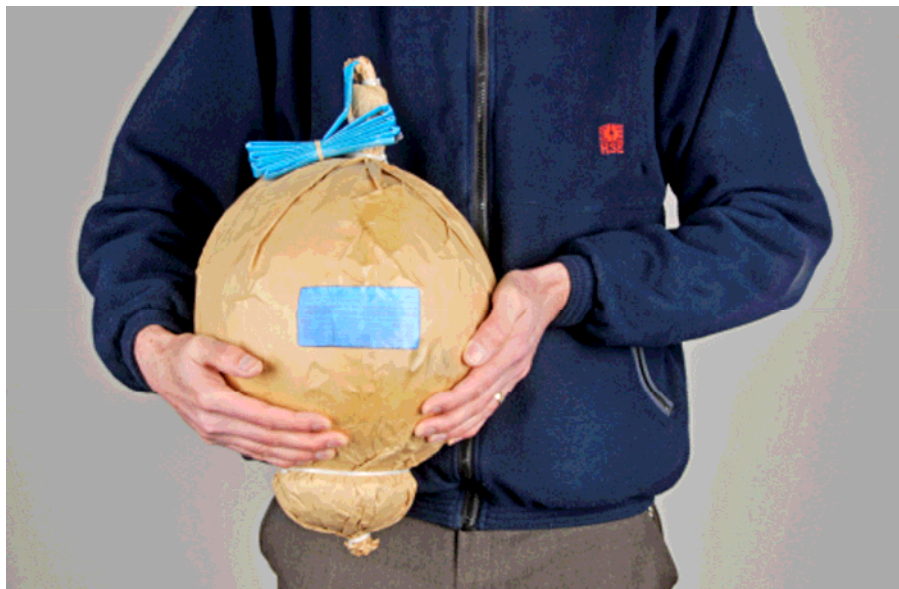
Mock up of 300mm shell found in magazine E post explosion (photo from HSE)
