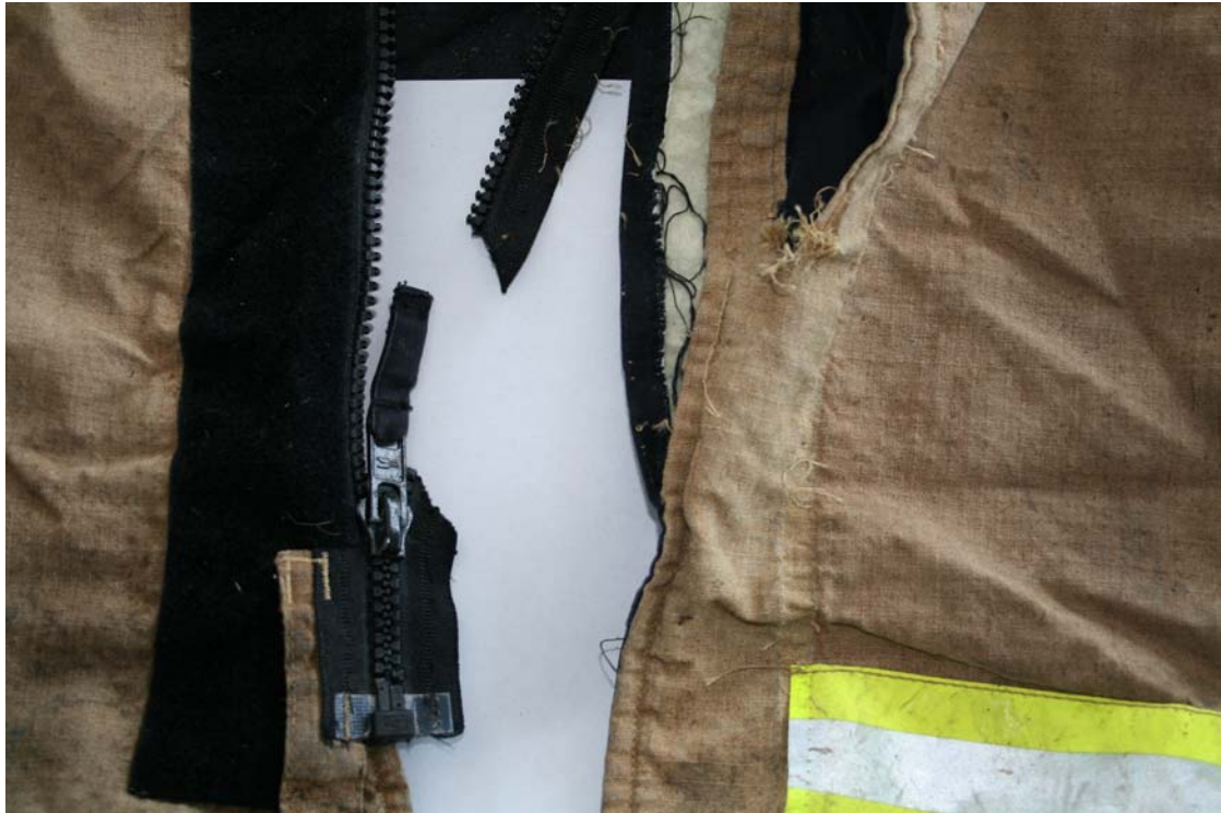
Damage to Tunic, note damage to Zip and total loss of covering flap
