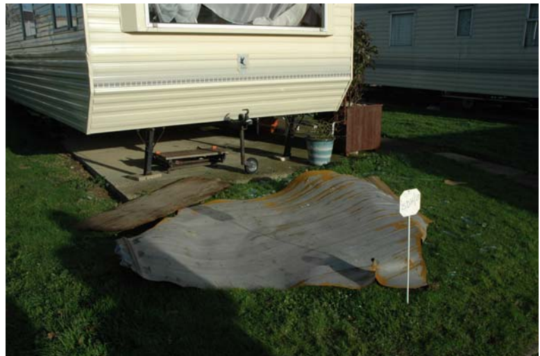
Section of ISO roof in caravan park 270 meters away
