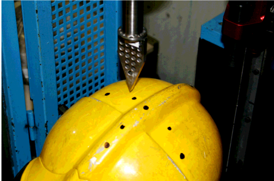
Impact testing of Gallet F1S/F1A helmet
