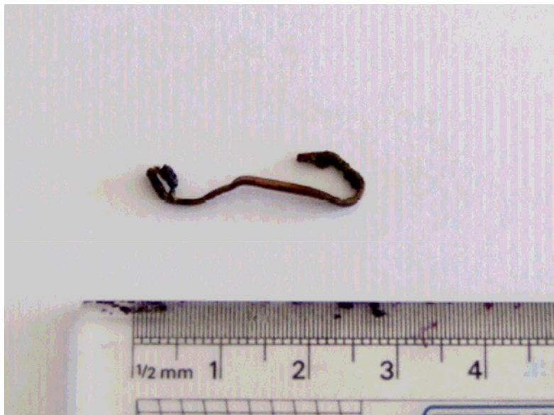
Metal fragment that penetrated overtrouser and subsequently removed from Firefighter's thigh in Hospital
