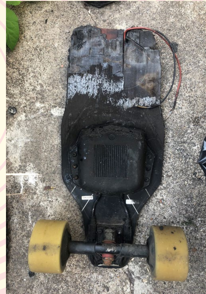
A damaged Electric skateboard that caught fire while stored under a bed in a child's bedroom.
