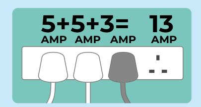
An extension lead or adaptor will have a limit to how many amps it can take, so be careful not to overload them to reduce the risk of a fire. Appliances use different amounts of power – a television may use a 3amp plug and a vacuum cleaner a 5amp plug for example.
